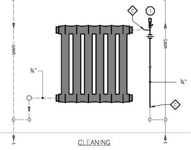
NEW AIR VENT WATTS MODEL HAV PROVIDED AND INSTALLED BY THE FOLLOWING CONTRACTOR. (AIR VENT INSTALLED DURING CLEANING PHASE; SAME AIR VENT AS IN ADJACENT CONSTRUCTION VIEW)
